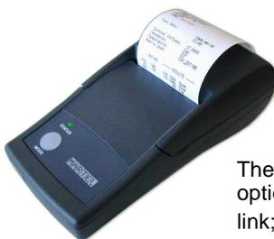
The CA-12 interfaces to optical printer by infrared link; prints test results.
